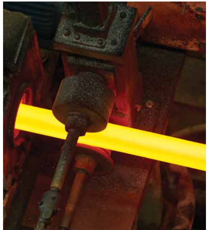
▲ BlueCoil® technology is a heat treated coiled tubing that is designed to last between two to four times longer than conventional coiled tubing.
