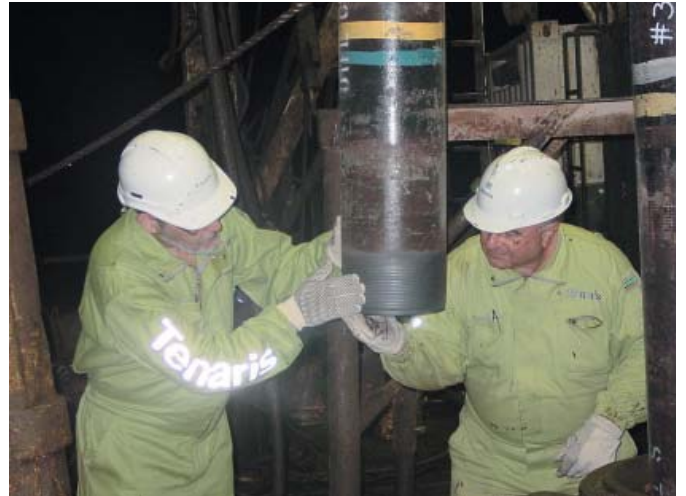
▲ Tenaris offered technical assistance, inspecting a TenarisHydril Blue™ Dopeless® connections before running.
