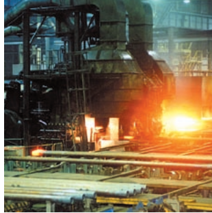
▲ Upsetting of drill pipe
