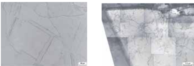
Fig.1 Microstructure of a tube ODxWT 50.8x10.3mm Left: Optical Microscope; Right: Transmission Electronic Microscope
