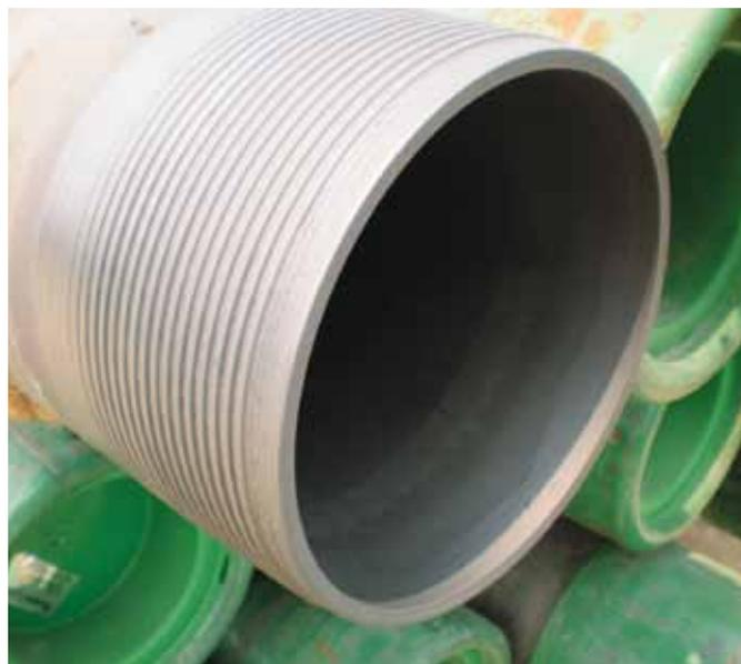
▲ Nearly 160 joints joints with Dopeless® technology were run in the 9 5/8" sections with no rejects.
