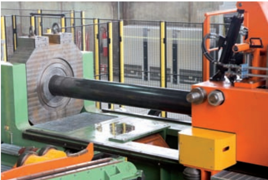
The 450-ton drawing bench installed at TenarisDalmine Costa Volpino plant.
