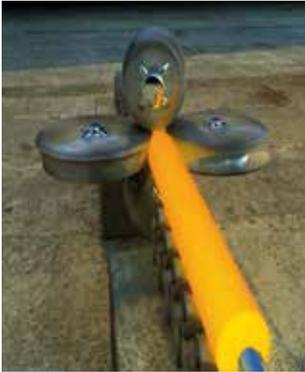
The Diescher mill, by means of transverse rolling, permits a hollow of lower wall thickness and even better concentricity to be obtained.
