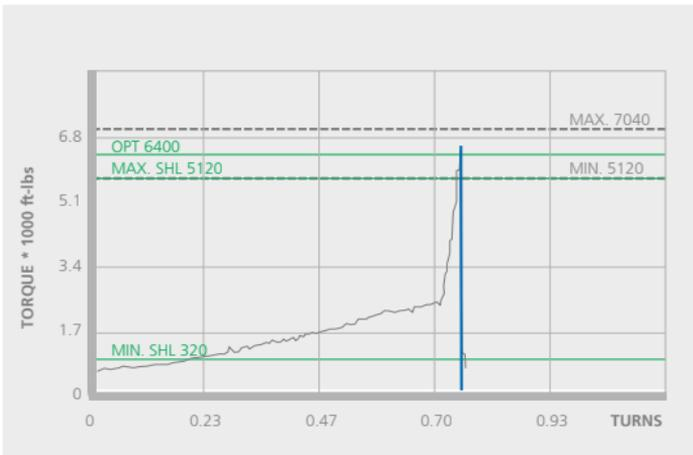
**10.** If 3SB™ is to be mixed with 3SB-ST™ the lower variant torque should be applied.
