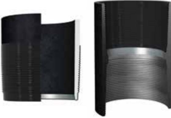
1. Apply a thin coating of thread compound on the pin and box connections, fully covering all threads, seals, pin nose and box torque shoulder, the thread form should be fully visible.
