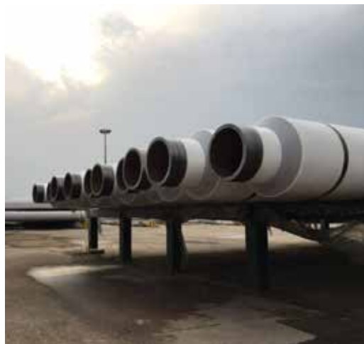
— Thermal Insulation and concrete weight coating.
