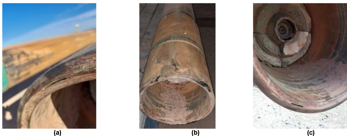
Figure 6—13 3/8" casing failure section, first well.
