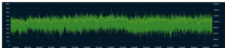
Figure 18—Torque from sensor compared to torque registered in a EDR – Casing drilling
