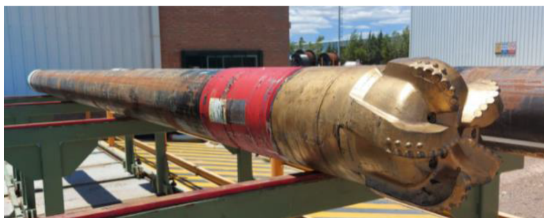
Figure 10—BHA configuration to improve stiffness and reduce bending stress magnification.
