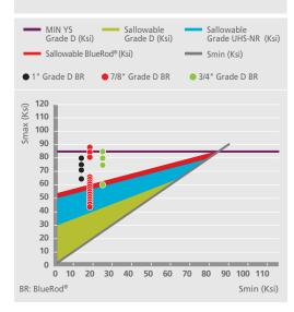
The connections' stress level was evaluated following the Modified Goodman Diagram method, as recommended by API Specs. Results showed that:
