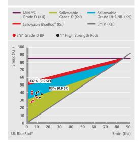
The chart shows 7/8" Grade D BlueRod® working under similar stress conditions to those of 1" high-strength rods with conventional connections. In this scenario, the new Tenaris BlueRod® has enabled a higher Grade D efficiency to be achieved in the field.
