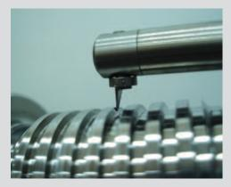
Tenaris uses state-of-the-art numerical control lathes and control gauges in order to ensure the highest quality in its connections.
