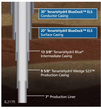
▲ TenarisHydril BlueDock™ connectors were used in both the conductor and surface casings of the Arima 2 well.
