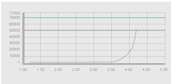
**19.** No shoulder will be evident in the graph, there should be a smooth thread & seal interference build profile culminating at optimum torque.
