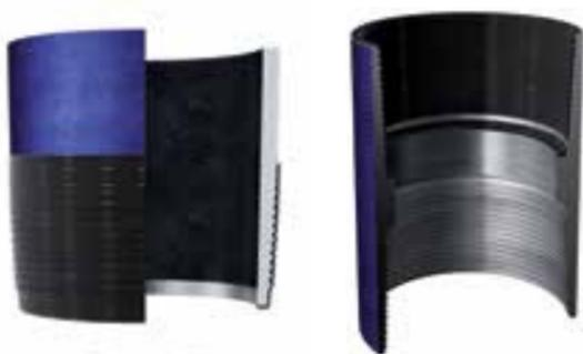
1. Apply a thin coating of thread compound on the pin and box connections, fully covering all threads, seals, pin nose and torque shoulders, the thread form should be fully visible.
