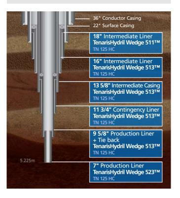
larger than that of the pipes used to case the well. With such tight clearances, casing joints risk becoming stuck in the formation.
