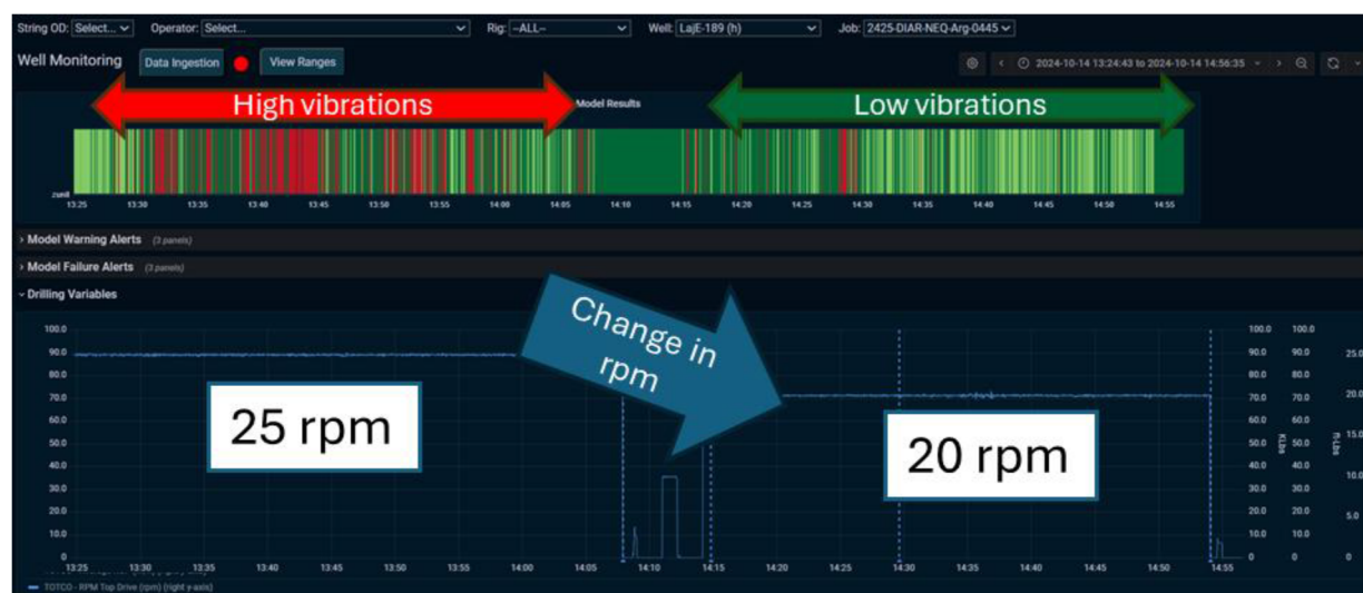
Figure 16—Screenshot of the Tenaris vibration monitoring application.
