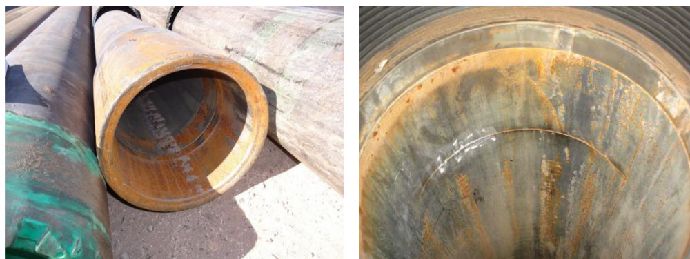
Figure 3—Failure of 9 5/8" TXP BTC during casing drilling operations (Well Laj-75) Tight gas development 2015 (Codega Dario, 2015).
