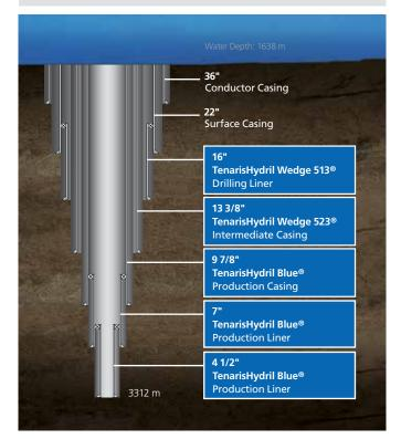
Vietgazprom ran TenarisHydril Blue®, Wedge 513® and Wedge 523® connections in the first deepwater well in Vietnam. The reverse angle stab flank of their threads ensures high compression ratings, making them suitable for the most severe compression applications. In addition, they come with 100% collapse rated metal-to-metal seal.
