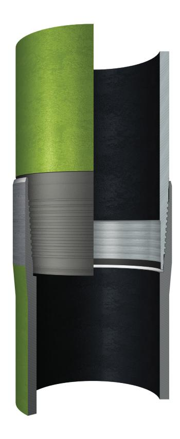
The TenarisHydril Wedge 624™ stems from the well-established TenarisHydril Wedge 623® connection, presenting greatest resistance to wear while maintaining the outstanding performance of the Wedge 623® connection. This product incorporates design elements that make the connection more robust, featuring an additional external metal-to-metal seal and offering unmatched compression ratings in an integral connection.
