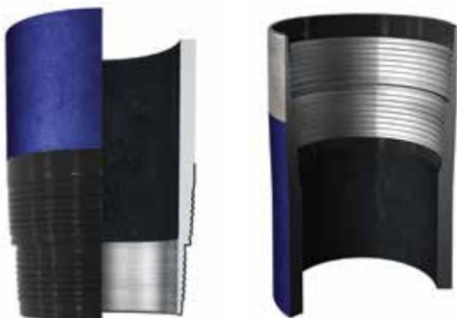
1. Apply a thin coating of thread compound on the pin connection, fully covering all threads, seals, pin nose and torque shoulder, the thread form should be fully visible.
