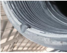
Damage inflicted to face and torque shoulder of a coupling during insertion of CRT grapples.
