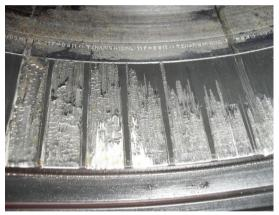
Gouging on pipe ID and across the coupling central area by insertion / removal of grapples.
