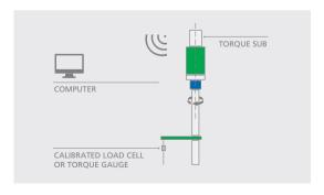
NOTE: VERIFY THE TOROUE READING FROM TOROUE SUB TO COMPUTER CORRESPONDS TO THAT INDICATED BY THE LOAD CELL.
