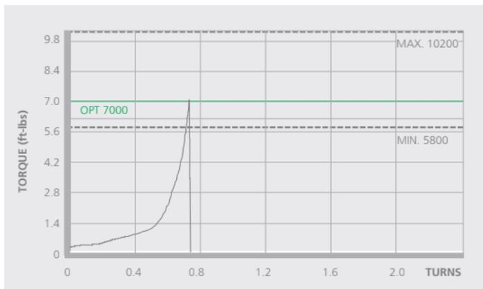
14. Wedge 563® has limited same size / weight interchange capability, if mixing weight / grade ensure compatibility of design and apply the higher torque value of the two connections.
