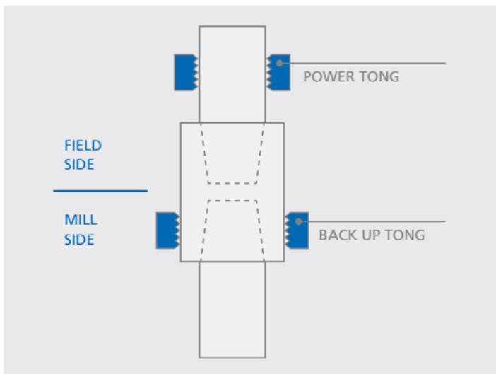
Tong positioning for breaking out of Blue® Series, Legacy Series, Wedge Series 400™ and TenarisXP® Buttress coupled connections.
