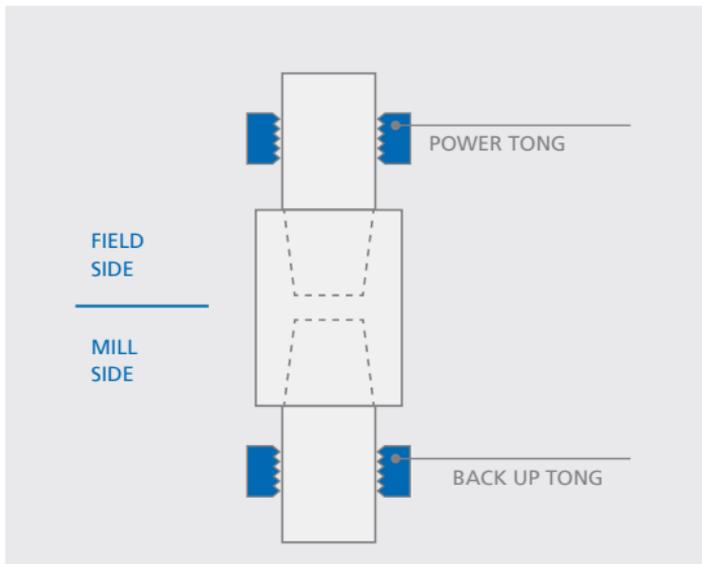
Tong positioning for break out of Wedge Series 500™ and Wedge series 600™ coupled connections.
