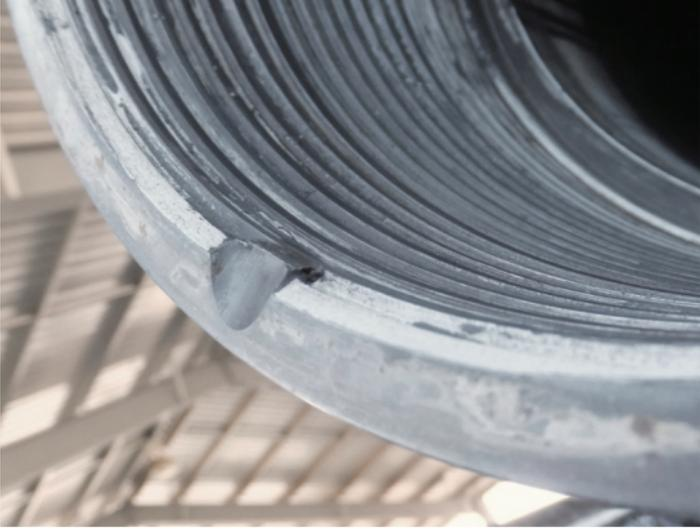
Damage inflicted to face and torque shoulder of a coupling during insertion of CRT grapples.
