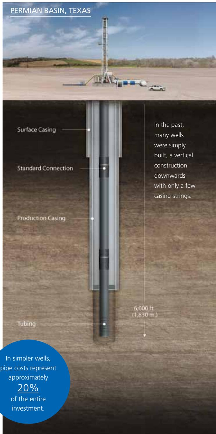
In the past, many wells were simply built, a vertical construction downwards with only a few casing strings.
