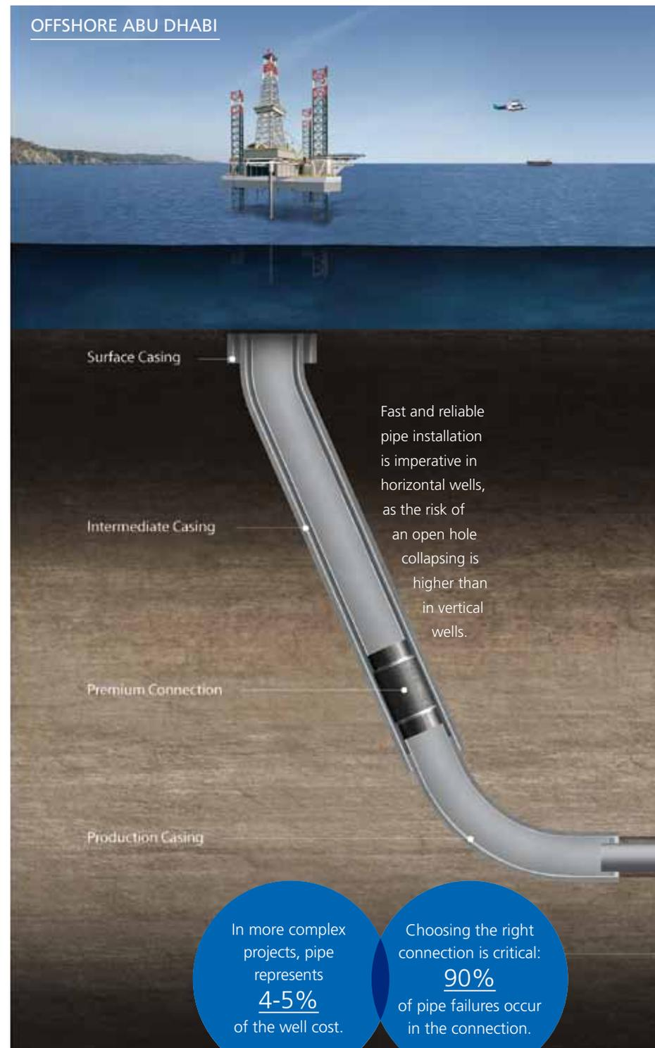
Fast and reliable pipe installation is imperative in horizontal wells, as the risk of an open hole collapsing is higher than in vertical wells.
