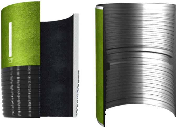
1. Apply a thin coating of thread compound on the full pin end only, threads and pin nose, the thread form should be clearly visible.
