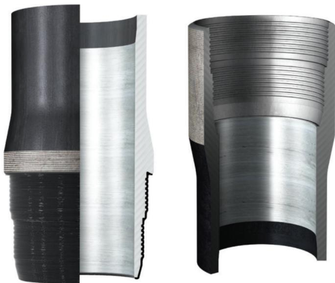
1. Apply a thin coating of thread compound on the full pin end only, threads, seals and pin nose, the thread form should be clearly visible.
