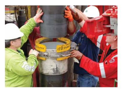
Once the well enters production, having Dopeless® technology brings additional benefits in terms of well productivity. This arises from the elimination of excess chemicals in the well bore, created by thread compounds during the assembly process.
