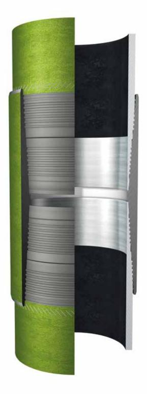
The TenarisHydril Wedge 667<sup>®</sup> connection was designed for HP/HT and deep well applications. With wear resistance in mind, it features two metal-to-metal seals. The two step profile with patented step-to-step Wedge provides exceptional high torque capability and locks the intermediate seal in place.
