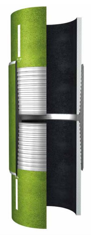
TenarisHydril Wedge 441™, designed for production casing in shales, has the slimmest OD in the market, comparable to that of an integral joint. The reduced coupling OD allows the use in clearance restricted applications. Additionally, the Wedge thread profile and shoulder back-up provides exceptional torque capability and robustness for handling rotation in longer laterals.
