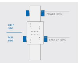
Tong positioning for breaking out of Blue® Series, Legacy Series, Wedge Series 400™ and TenarisXP® Buttress coupled connections.
