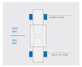
Tong positioning for break out of Wedge Series 500<sup>™</sup> and Wedge series 600<sup>™</sup> coupled connections. **6.** Never grip the connection OD of any integral connection.
