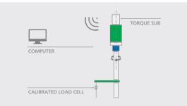
NOTE: VERIFY THE TORQUE READING FROM TORQUE SUB TO COMPUTER CORRESPONDS TO THAT INDICATED BY THE LOAD CELL
