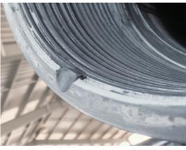
Damage inflicted to face and torque shoulder of a coupling during insertion of CRT grapples.
