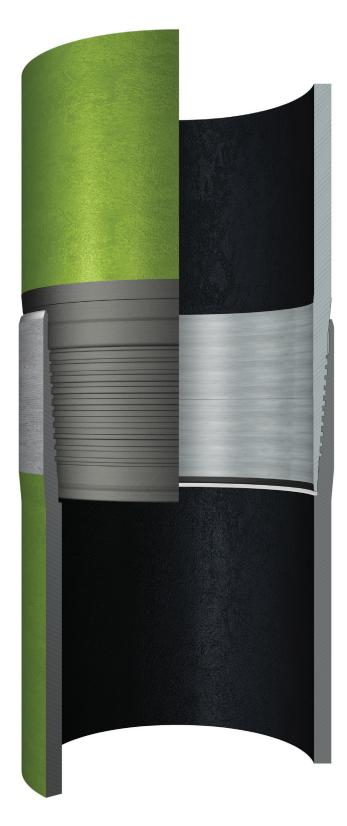
The TenarisHydril Wedge 623<sup>®</sup> connection was developed to comply with recent changes in deepwater operating requirements in the Gulf of Mexico. The new connection is an improved version of the Wedge 523<sup>®</sup> connection design featuring an additional external metal-to-metal seal and offering unmatched compression ratings (70-75% efficiency) in an integral connection.
