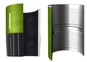
**1.** Apply a thin coating of thread compound on the full pin end only, threads and pin nose, the thread form should be clearly visible.
